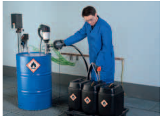
Semi-automatic can filling in explosion zone 1.
